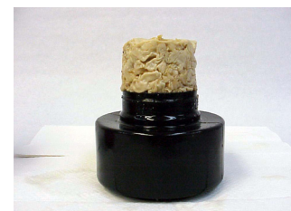
Individual pellet capsules after 50,000 miles of use meld into a single, gelatinous clod blocking the flow of coolant through the filter.
