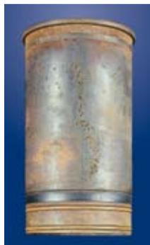
A cylinder liner destroyed by cavitation-erosion
